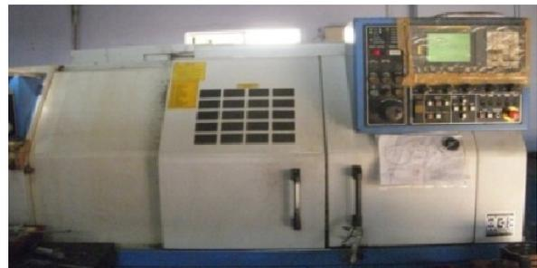
**Figure 1:** CNC Lathe Used for Machining.
