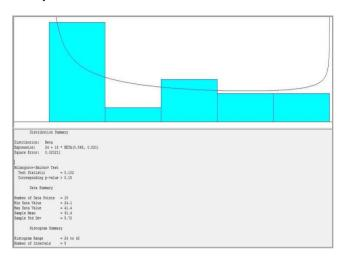
Figure 3: Input analyzer data distribution function window for Back Lasting Operation
