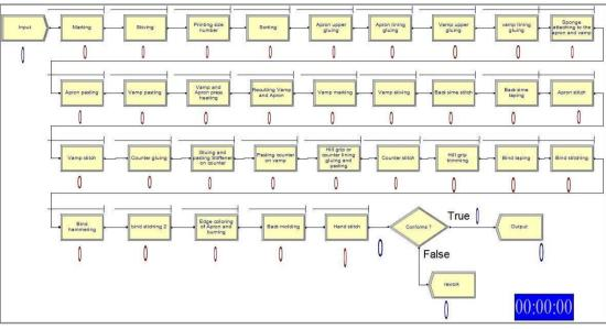
Figure 8: Proposed stitching assembly line simulation model for scenario 1 and 2
