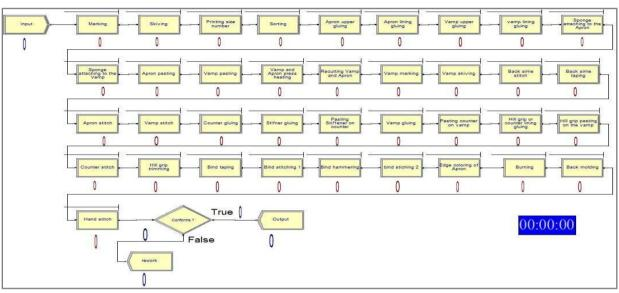
Figure 4: Stitching assembly line simulation model for existing manufacturing system
