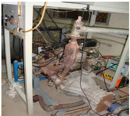
Figure 5: Experimental setup with electrically heated metal. Cataly11c (EHMC) converter.
