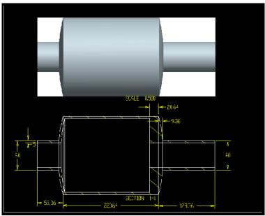
Figure 2: Outer design of converter.
