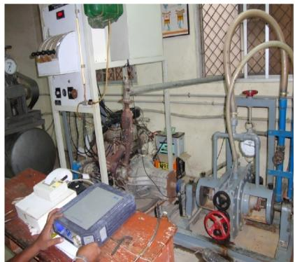
Figure 6: Performance of electrically heated metal. Catalyt1c (EHMC) converter with emission test set up.
