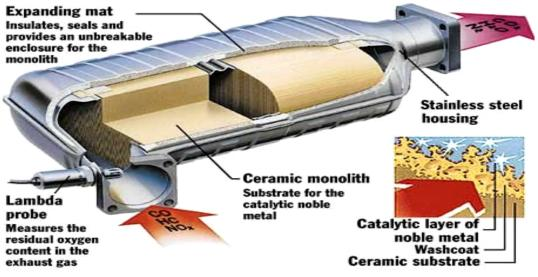
Figure 4: Structure of Catalytic converter.
