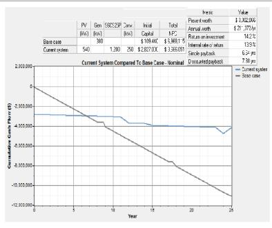
Figure 9: Economic comparisons of SAPV system and Diesel-only system.
