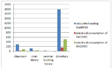
Figure 3: Cooling load & electric consumption of air conditioning system.
