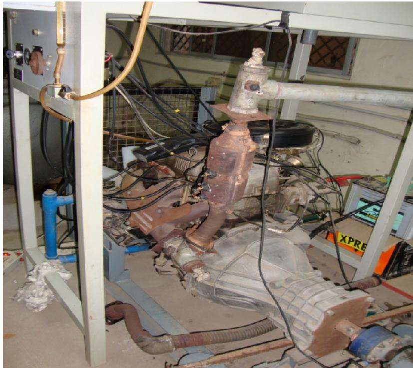
**Figure 5:** Experimental setup with electrically heated metal. Catalytic converter (EHMC) converter.
