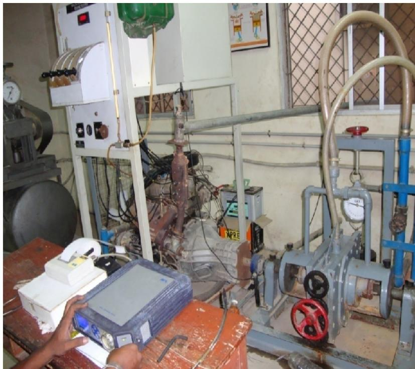
**Figure 6:** Performance of electrically heated metal. Catalytic converter (EHMC) converter with emission test set up.
