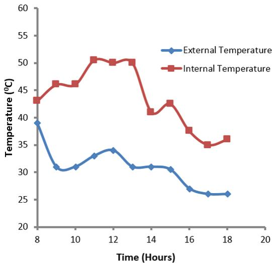
Fig. 5: Hourly variation of external and internal temperatures (Day 3)
