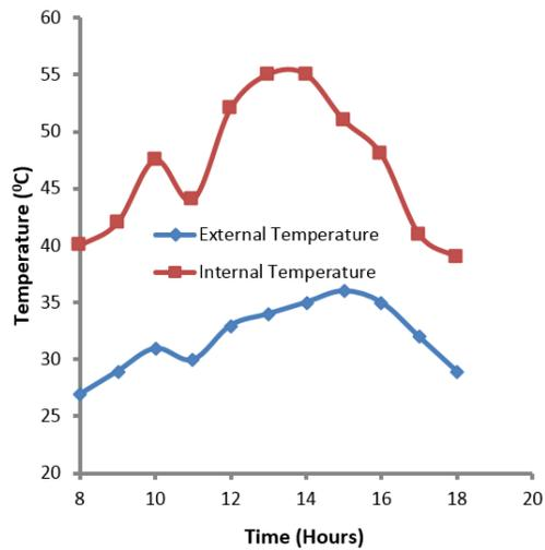
Fig. 8: Hourly variation of external and internal temperatures (Day 6)
