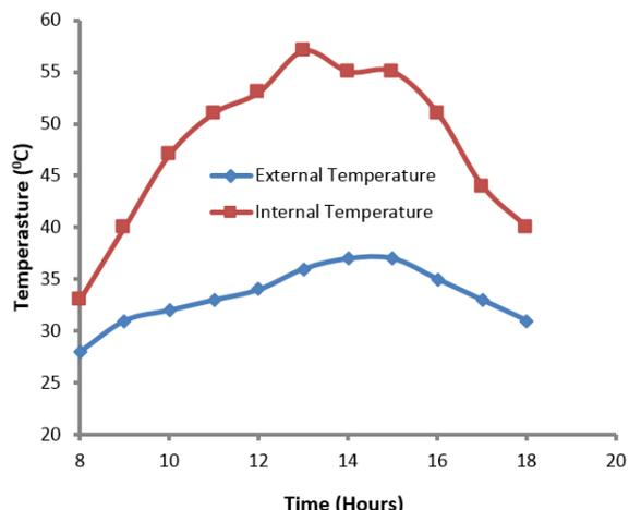
Fig. 9. Hourly variation of external and internal temperatures (Day 7)
