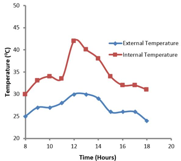
Fig. 7: Hourly variation of external and internal temperatures (Day 5)
