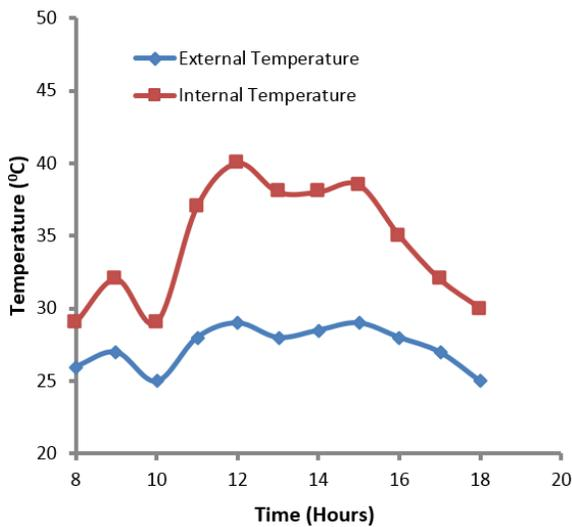
Fig. 4: Hourly variation of external and internal temperatures (Day 2)
