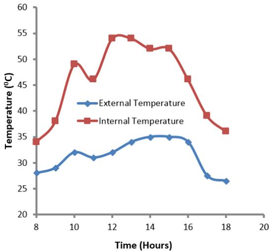
Fig. 3: Hourly variation of external and internal temperatures (Day 1)
