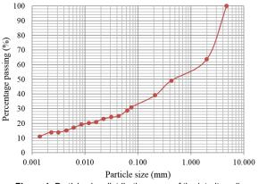
Figure 1: Particle size distribution curve of the laterite soil Table 1: Index properties of laterite soil
