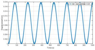
Figure 2: Effect of Non -local parameter at 0.31nm on deflection of the pipe
