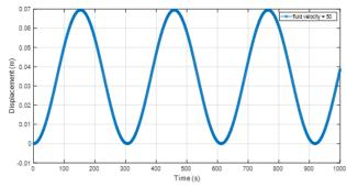
Figure 6: Effect of fluid velocity at 50m/s on deflection of the pipe
