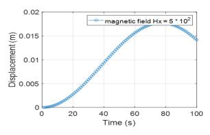
**Figure 5:** Effect of magnetic field at  $5 \times 10^2 A/m$  on deflection of the pipe
