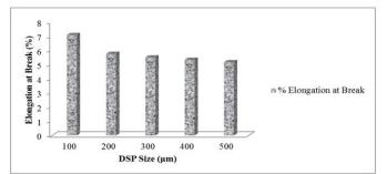
Figure 3: Effect of Particle Size on Elongation at Break of DSP-UPR Composites
