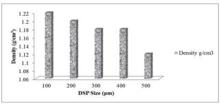
Figure 4: Effects of Particle Size on Densities of UPR-DSP Composites
