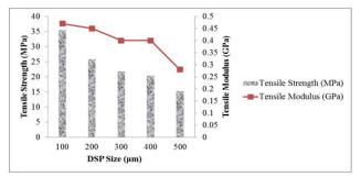
Figure 2: Effect of Particle Size on Tensile Strength and Modulus of DSP-UPR Composites
