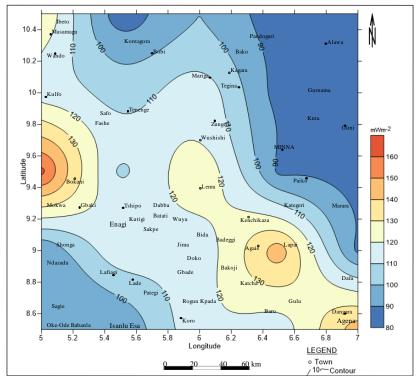
Figure.8: Heat Flow Map of Northern Bida Basin and Environs (Contour interval = 10 mWm<sup>-2</sup>)
