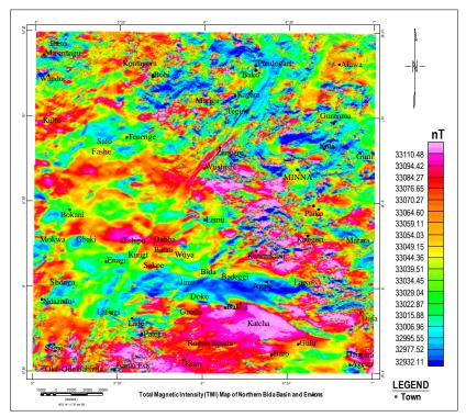
Figure. 2: Total Magnetic Intensity (TMI) Map of Northern Bida Basin and Environ (Adopted from Barka, 2020)
