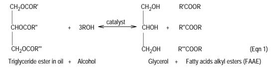
The choice of the catalyst and the nature of the alcohol determine the type of initial specie(s) and the nature of FAAE to be formed. In this study, the homogeneous reaction involved an initial separate interaction between KOH and NaOH with ethanol producing potassium ethoxide and sodium ethoxide (Equations 2 and 3) respectively.
