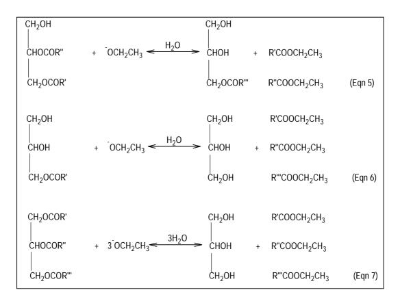
In the heterogeneous reaction three initial ethanol, oil and  $CaO/Al_2O_3$  layers were formed. With constant stirring the ethanol interacts with basic sites of calcium oxide to form surface ethoxide anioins (Equation 8) due to proton extraction from the hydroxyl group of ethanol (Liu *et al.*, 2008). These ionic species generated react with the oil in steps similar to those reported in equations 5 to
