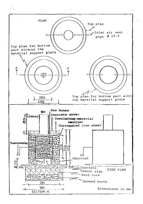
Figure 1: Low cost kiln for bones activation by heat treatment.
