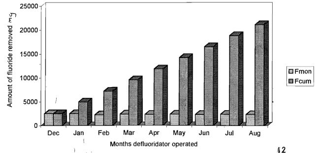
Monthly and cumulative fluoride removed as function of operating **Figure 3:** time.
