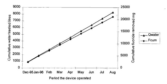
Figure 4: The amount of fluoride removed land accumulated in the filter column and quantity of water treated by the unit as function of operating time.
