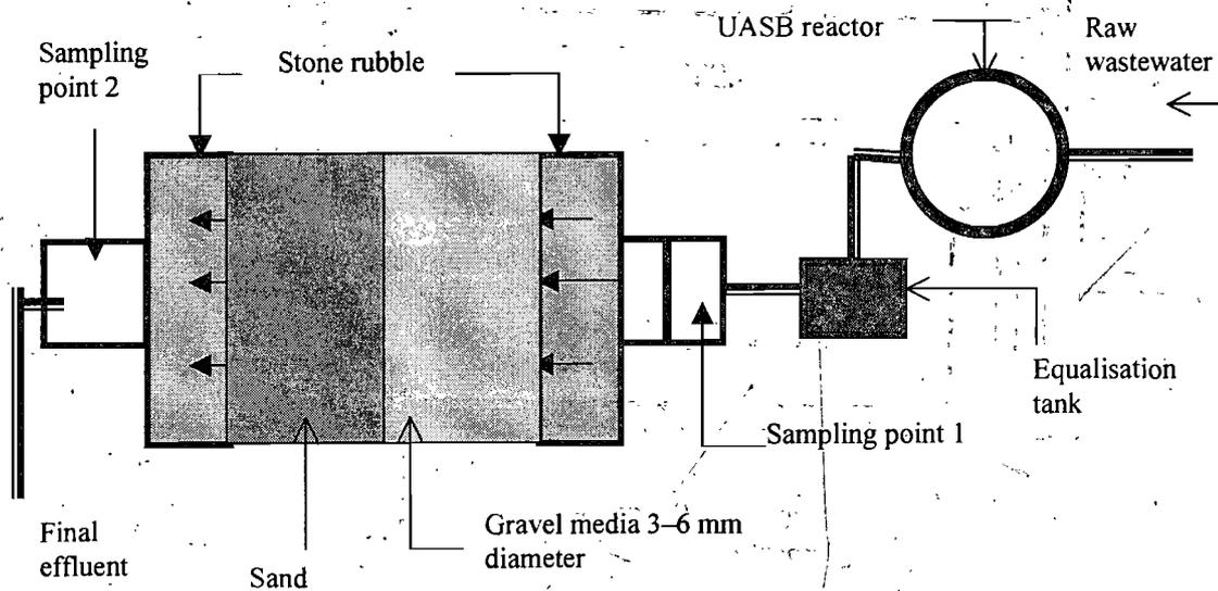
Figure 2(a): Schematic presentation of the experimental set up (plan)
