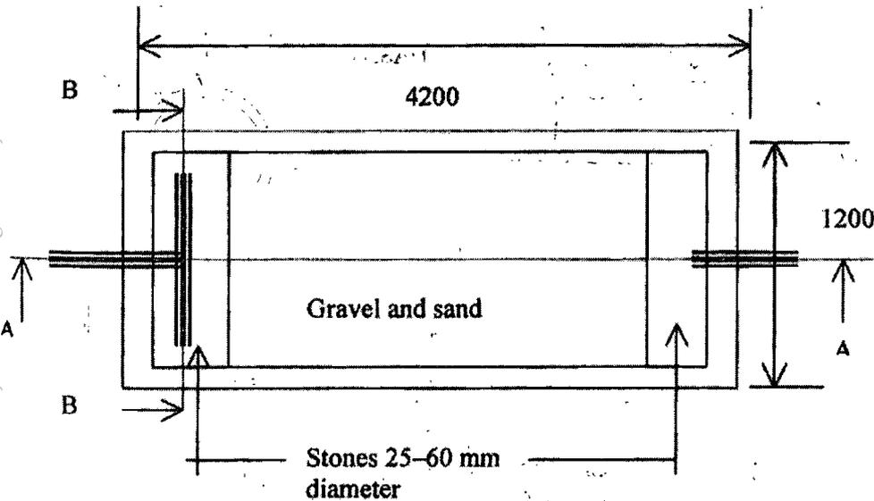
Figure 1(a): Schematic plan of a HSSFCW unit
