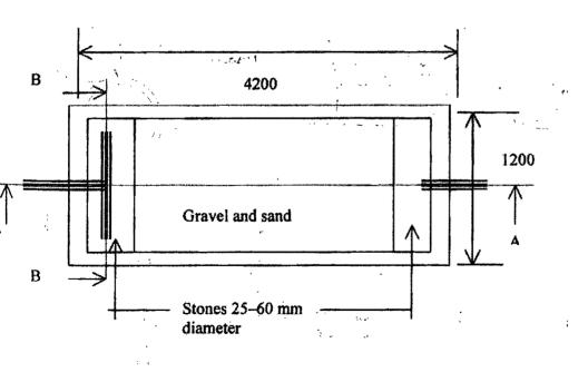
Figure 1(a): Schematic plan of a HSSCW unit
