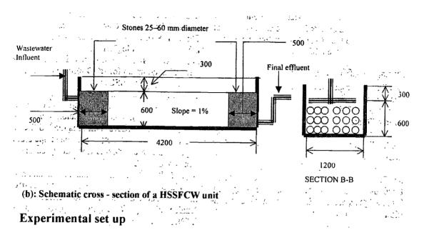
The experimental set up that was used is shown in Figure 2. A UASB and HSSFCW wastewater flow arrangement in which the HSSFCW unit was planted with *Typha latifolia* and packed with gravel (varying between 3 mm to 6 mm diameter) and sand was studied.
