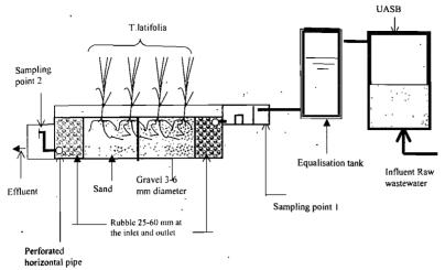
Figure 2(b): Schematic cross -section of the experimental set-up.
