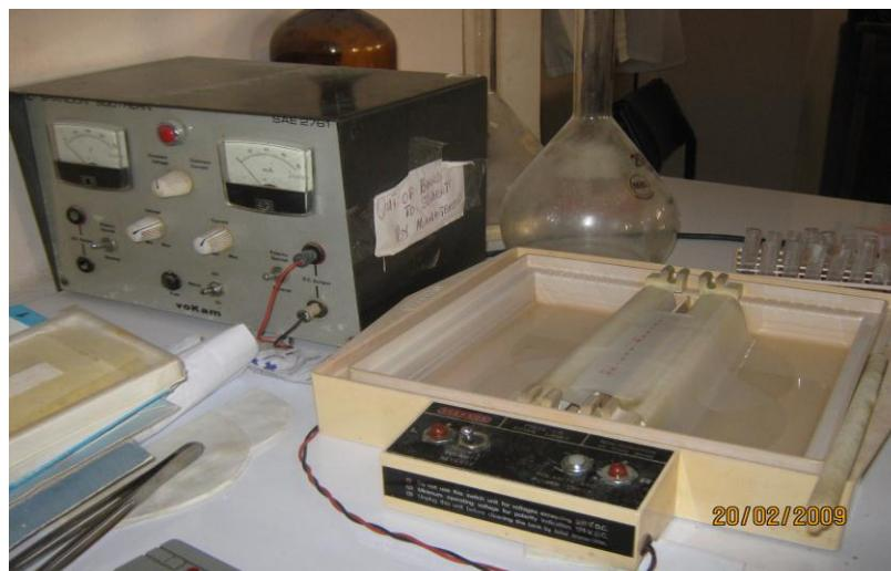
Fig 3- An electrophoresis tank with galvanometer
