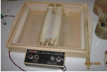
Fig 2- An electrophoresis tank showing acetate strips and band separations as a result of current flowing from a galvanometer.
