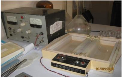
Fig 3- An electrophoresis tank with galvanometer
