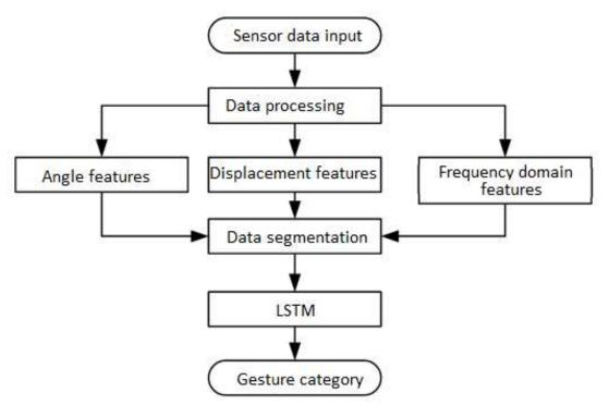
Figure 4: Flow chart of real-time hand gesture recognition
