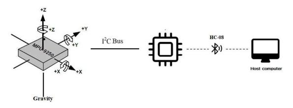
Figure 1: Schematic of hand-held somatosensory stick
