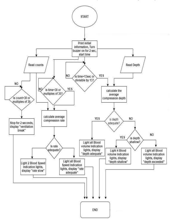
Figure 3: System Flow Chart of the proposed manikin.
