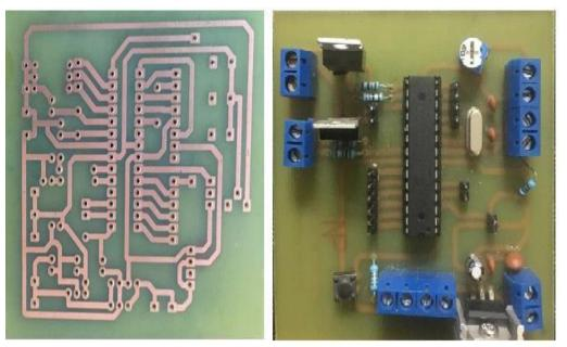
Figure 6: Printed circuit and device mounted on the board.
