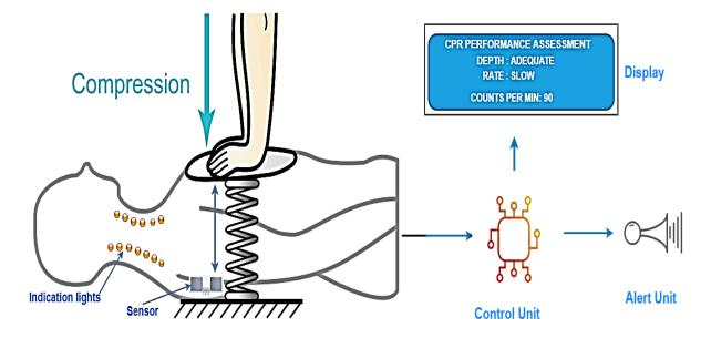
Figure 2: Conceptual diagram of a manikin model.
