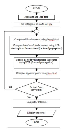
Figure 3: Flowchart of backward-forward sweep load flow algorithm.
