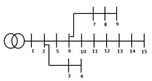
Figure 2: One line diagram of the Nigerian 11 kV network.
