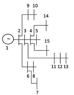
Figure 1: One line diagram of IEEE 15-bus RDS.
