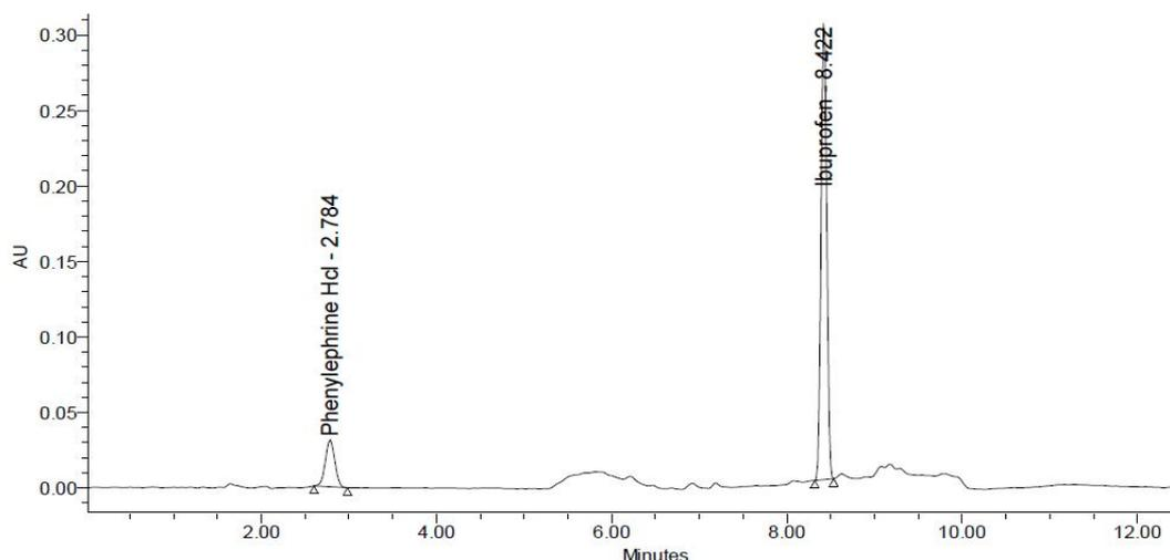
**Figure 2:** Representative chromatogram of phenylephrine and ibuprofen
