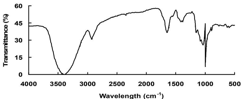
**Figure 3:** Fourier transforms infrared spectrometry of CEDs
