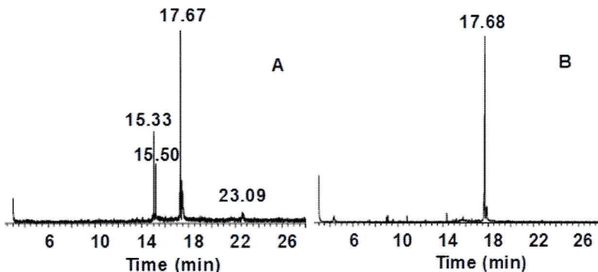
**Figure 2:** **A** = Gas chromatogram (GC) of CED monosaccharide standard (elution time for monosaccharides: 15.33 min, arabinose; 15.50 min, xylose; 17.67 min, glucose; 23.09 min, glucuronic acid); and **B** = GC profile of hydrolyzed CED polysaccharide hydrolyzate
