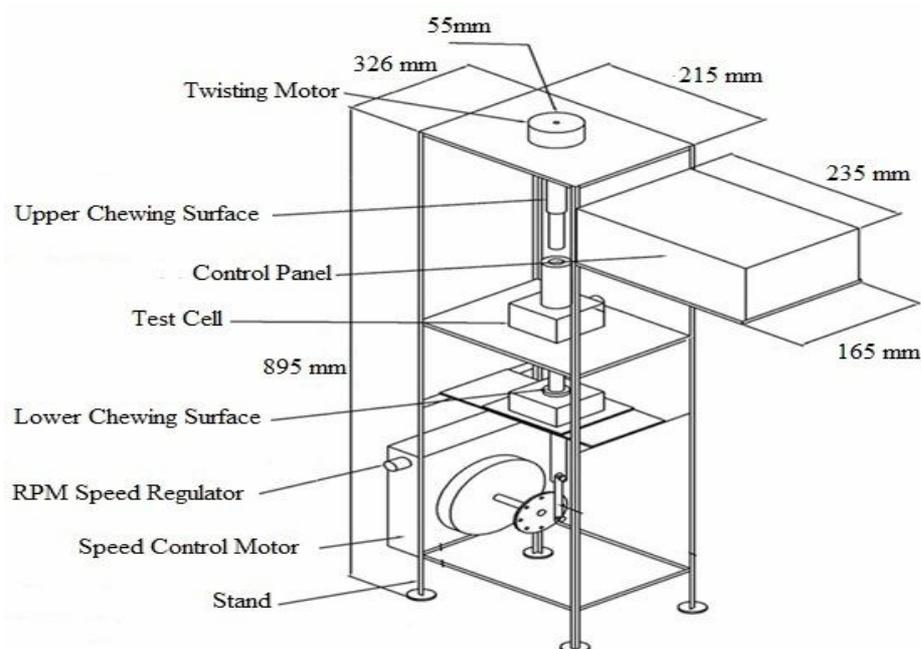
**Figure 2:** A sketch of the cross sectional view of *in vitro* chewing apparatus
