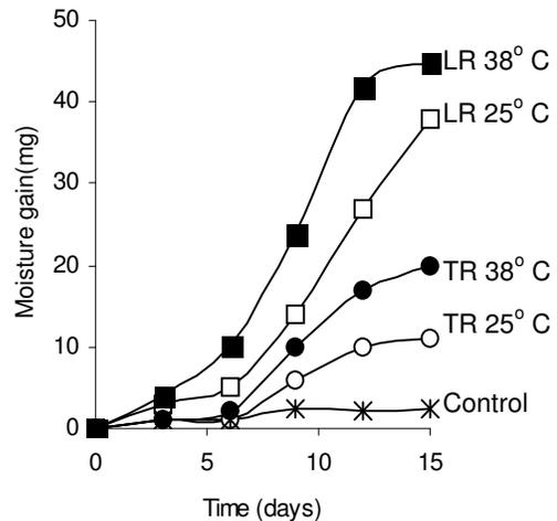
**Figure 2:** Reclosure efficiency of aspirin container under different conditions
