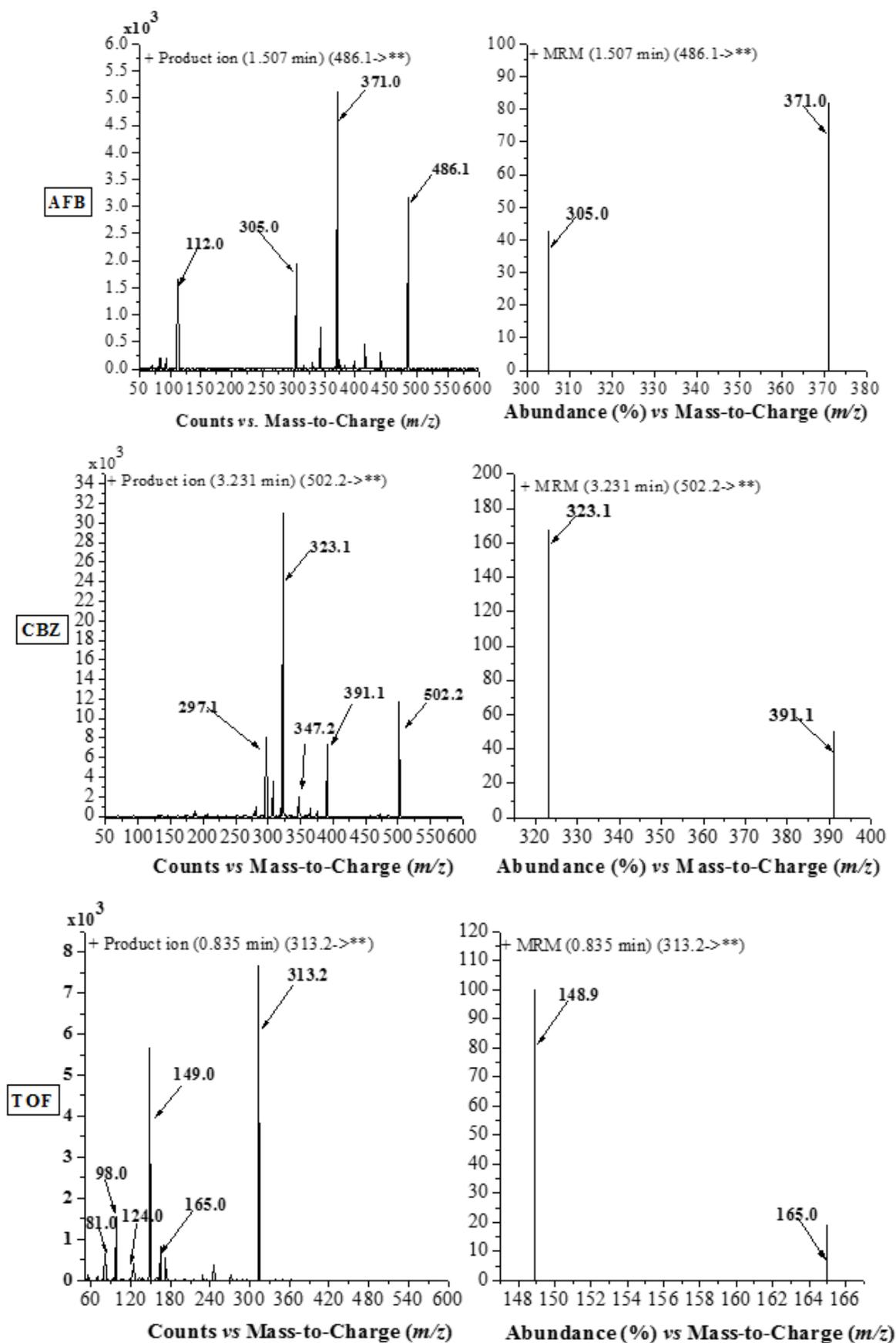
Figure 3: MS<sup>2</sup> and MRM spectra of TOF, AFB, and CBZ.
