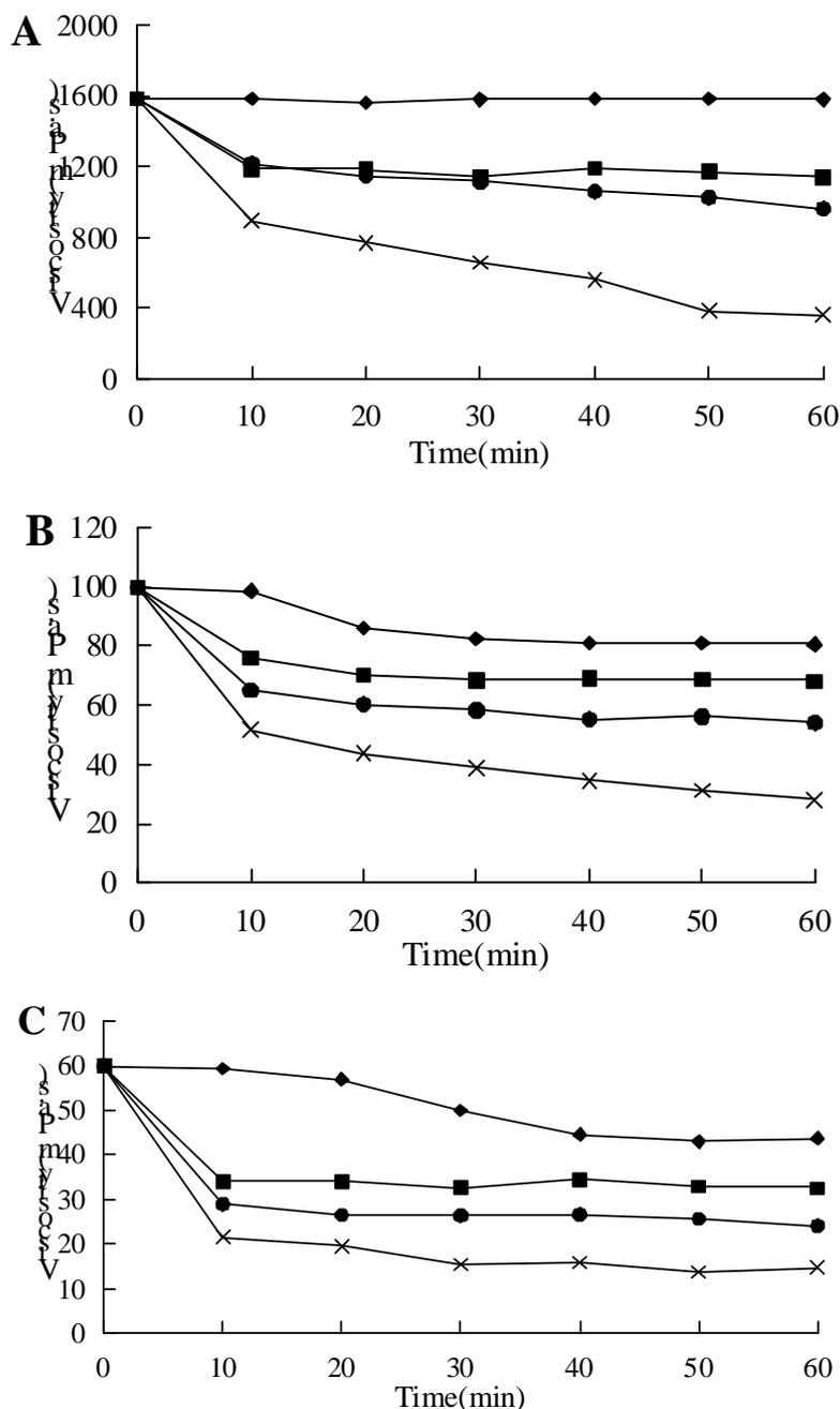
**Figure 3:** Effect of temperature and dilution on broth viscosity. Culture broth diluted 2-fold (A); culture broth diluted 3-fold (B); culture broth diluted 5-fold (C). **Note:** ◆ = fermentation broth was treated at 35 °C; ■ = fermentation broth was treated at 45 °C; ● = fermentation broth was treated at 55 °C. × = fermentation broth was treated at 65 °C
