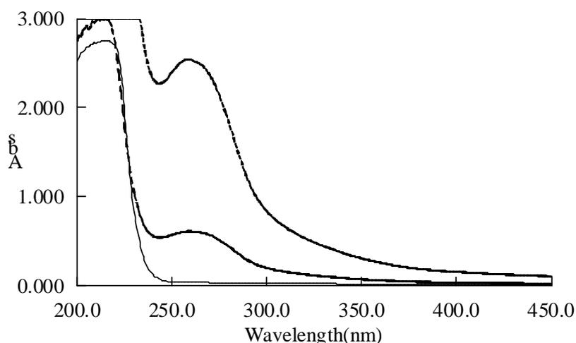
**Figure 5:** Spectral analysis of the culture broth (treated and untreated with activated carbon), and high purity  $\gamma$ -PGA over wavelength range of 200 to 500 nm. **Note:** From top to bottom, the curves represent treated and untreated with activated carbon, high purity  $\gamma$ -PGA.
