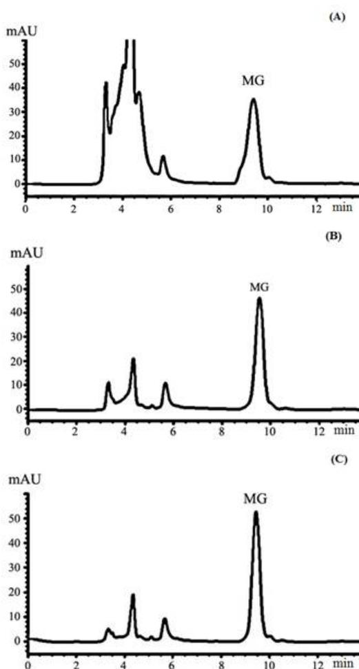
**Figure 2:** Chromatograms of MG after passing the cartridges with methanol-water mixture containing 2 % ammonium hydroxide; (A) single passing with 5 % methanol; (B) single passing with 70 % methanol; (C) double passing with 5 % followed by 70 % methanol
