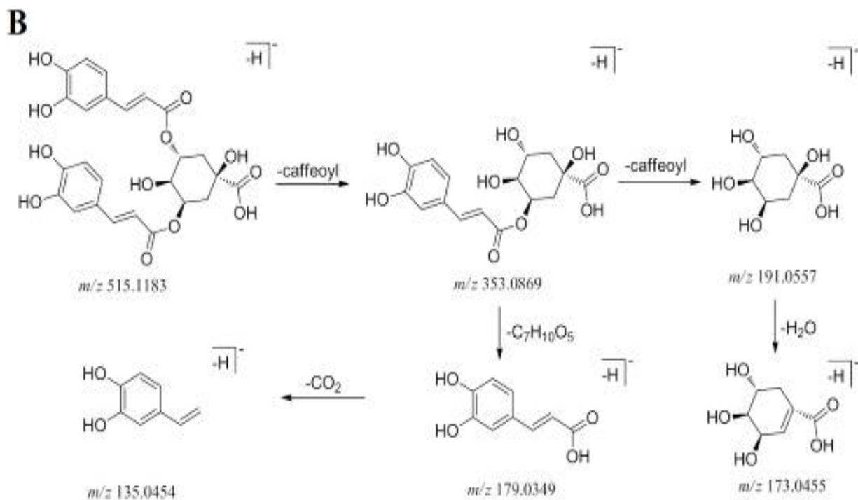
**Figure 4:** MS diagram (ESI<sup>-</sup>) and ions fragmentation pathways of 3,5-dicafeoylquinic acid (16)
