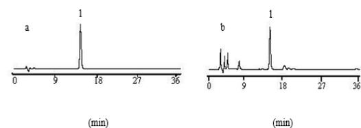
**Figure 1:** Chromatogram of ferulic acid standard (a), and *chuanxiong* sample (b).
