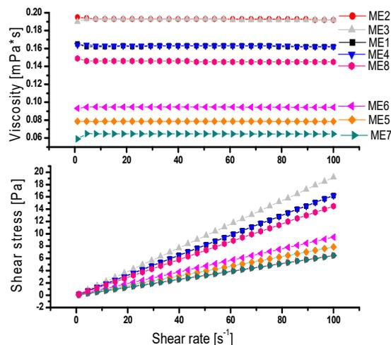
**Figure 2:** Rheograms of different MEs: the shear rate against viscosity and shear rate against the shear stress
