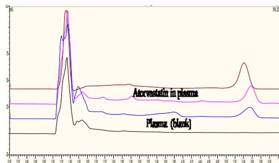
**Figure 5:** Chromatograms for extracted blank plasma and plasma after application of atorvastatin using high pressure liquid chromatography (HPLC)
