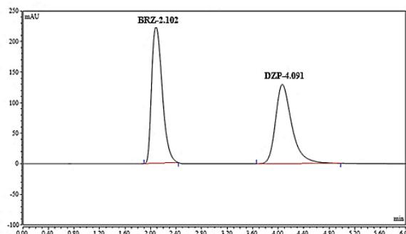
**Figure 2:** The UPL chromatogram for the separation pattern of a mixture of BRZ and DZP
