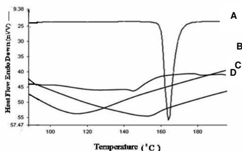
**Fig 4:** DSC thermograms of pure indomethacin (A) and chitosan films (B = F6, C = F11, and D = F1) (Code key as in Table 1)
