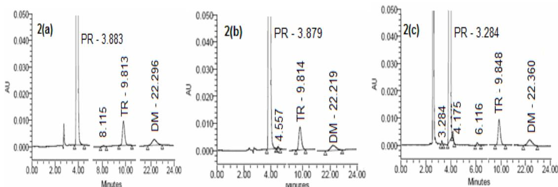
**Fig 2:** Typical LC chromatograms of a sample obtained after (a) acid degradation (b) base degradation and (c) peroxide degradation
