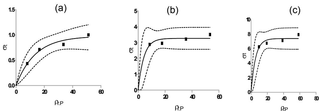
**Figure 2:** Plot of radial crushing strength against the product of pressure of compression pressure and relative density of *Saraca indica* bark for (a) powder (b) direct compression formulation, and (c) granules
