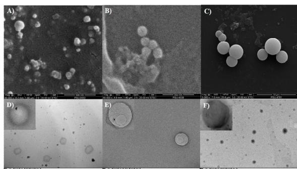
**Figure 6:** SEM photographs of ethosome (A), transfersome (B) and invasome formulations (C), and TEM photographs of ethosome (D), transfersome (E) and invasome formulations (F), respectively
