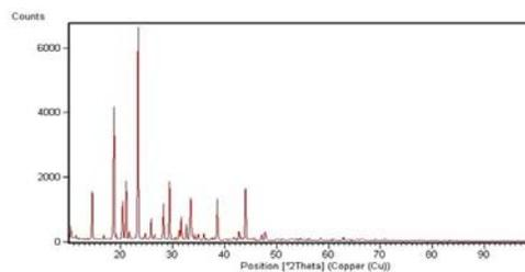
**Figure 3:** X-ray powder diffraction patterns of mannitol pure powders
