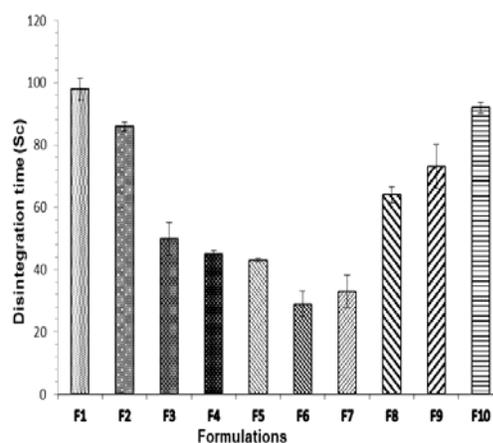
**Figure 9:** Effect of Starch (F1-F5) and MCC (F6-F10) concentrations (5-70% w/w) on the disintegration time of binary mixture tablets. Tablets were compressed at 3 tonnes compression force. Results reported as mean  $\pm$  SD (n = 3)
