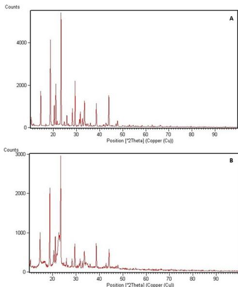
**Figure 7:** X-ray powder diffraction patterns of (A) 5 % w/w MCC interactive mix and (B) 70 % w/w MCC interactive mix
