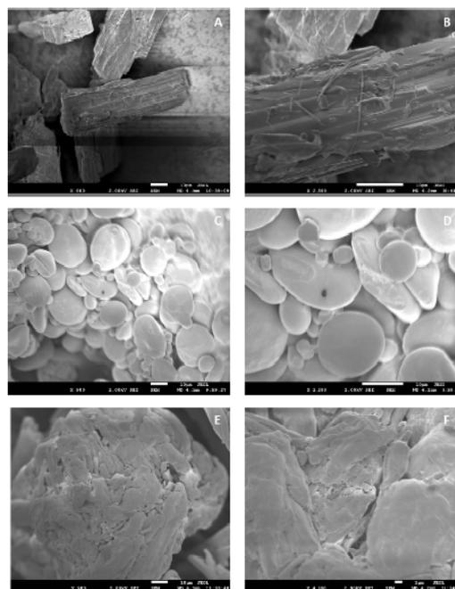
**Figure 1:** Scanning electron micrographs (x300 and 2500) magnification for (A and B) mannitol, (C and D) starch and (E and F) MCC powders
