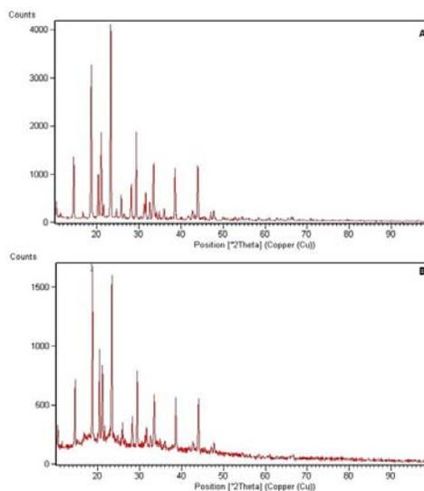
**Figure 6:** X-ray powder diffraction patterns of (A) 5 % w/w starch interactive mix, (B) 70 % w/w starch interactive mix
