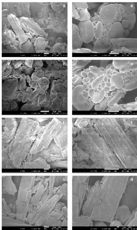
**Figure 2:** Scanning electron micrograph (x300 and 2500) magnification for (A and B) 5% starch mix, (C and D) 70% starch mix, (E and F) 5 %w/w MCC mix and (G and H) 70% w/w MCC mix
