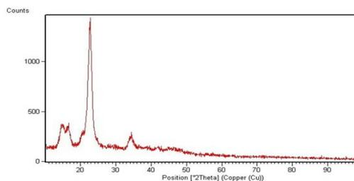
**Figure 5:** X-ray powder diffraction patterns of MCC pure powders
