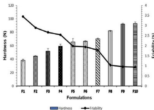
**Figure 8:** Effect of starch (F1 - F5) and MCC (F6 - F10) concentrations (5-70% w/w) on hardness and friability of binary mixture tablets. Tablets were compressed at 3 tonnes compression force. Results of hardness reported as mean  $\pm$  SD (n=3)
