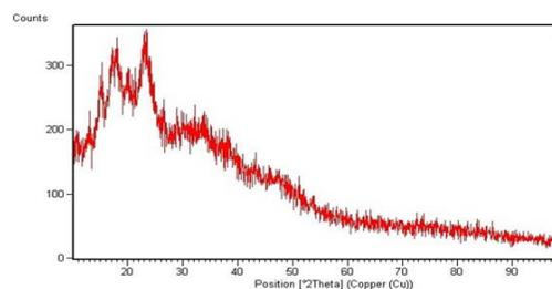
**Figure 4:** X-ray powder diffraction patterns of starch pure powders
