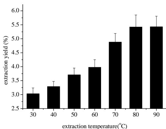
**Figure 1:** Effect of extraction temperature on yield of total flavonoids from *Drynaria* rhizome
