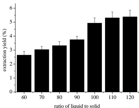
**Figure 3:** Effect of liquid: solid ratio on yield of total flavonoids from *Drynaria* rhizome
