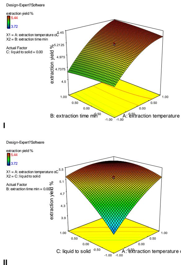
**Figure 4:** Response surface and contour plots showing the interaction effects of (I) A and B, (II) A and C on the extraction yield of total flavonoids from *Drynaria* rhizome. A: extraction temperature; B: extraction time; C: liquid: solid ratio
