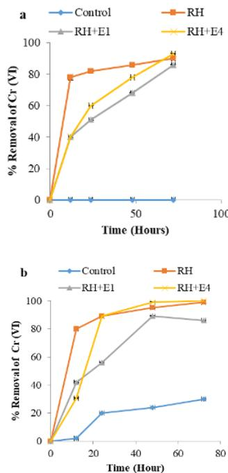
**Figure 2:** Elimination of Chromium VI from effluent with RH (a) sterile and (b) non-sterile
