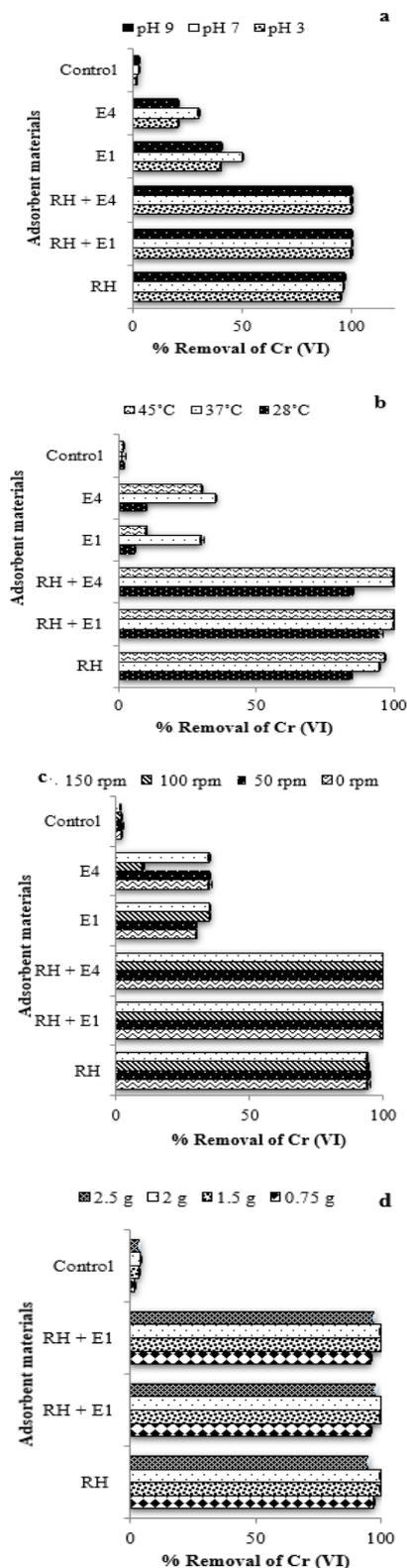
**Figure 1:** Investigations on optimum physical factors (a) variable pH (b) variable temperature (c) variable shaking speed (d) variable rice husk concentration
