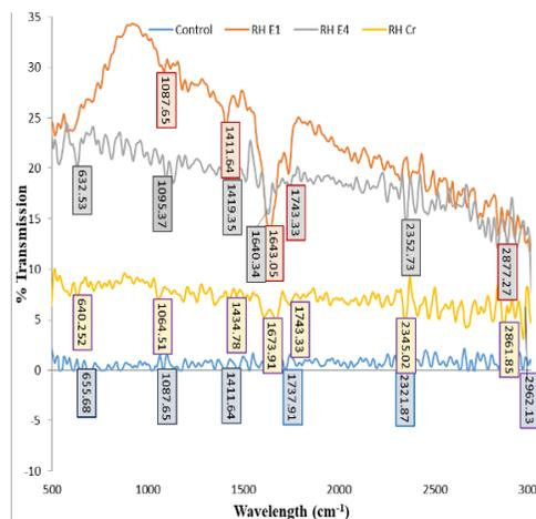
**Figure 3:** FTIR spectra of processed and unprocessed RH
