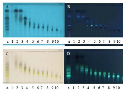
**Figure 1:** TLC profile of sub-fraction EA.1 – EA.12 (stationary phase: Silica RP-18). (a) EA fraction; (1 – 12) sub-fraction EA.1 – EA.12; (A) UV 254 nm; (B) UV 366 nm; (C) Visible; (D) UV 366 nm after spraying
