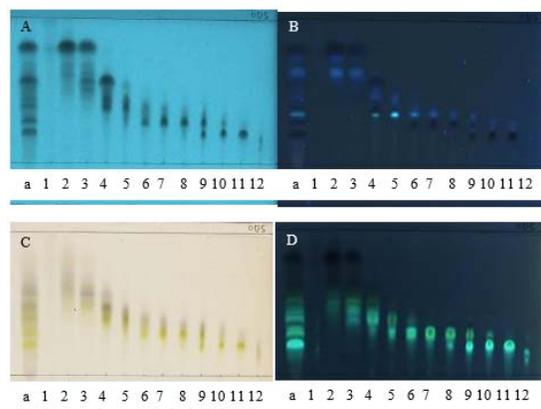
**Figure 2:** Chromatogram profile of sub-fractions ETA.1 – ETA.12 (stationary phase: Silica RP-18). (a) ETA fraction; (1 – 12) sub-fractions ETA.1 – ETA.12; (A) UV 254 nm; (B) UV 366 nm; (C) Visible; (D) UV 366 nm after spraying
