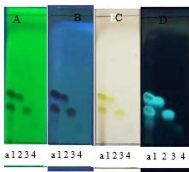
**Figure 3:** Chromatogram profile of sub-fractions ETA.11.1 – ETA.11.2 (stationary phase: Silica GF<sub>254nm</sub>). (a) ETA.11; (1 – 4) sub-fractions ETA.11.1 – ETA.11.4 (A) UV 254 nm; (B) UV 366 nm; (C) Visible; (D) UV 366 nm after spraying
