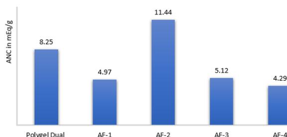
**Figure 3:** Acid-neutralizing capacity (ANC) of each of the products studied
