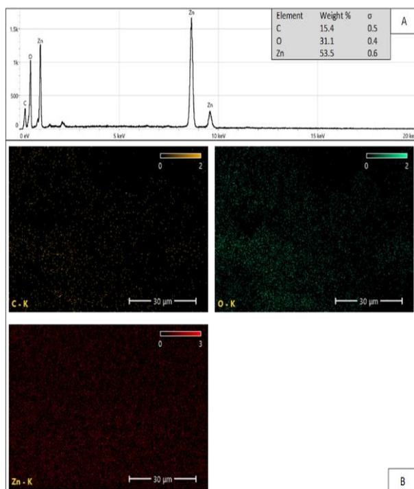
**Figure 6:** EDS (A) and elemental mapping (B) of the optimum formula (T25)
