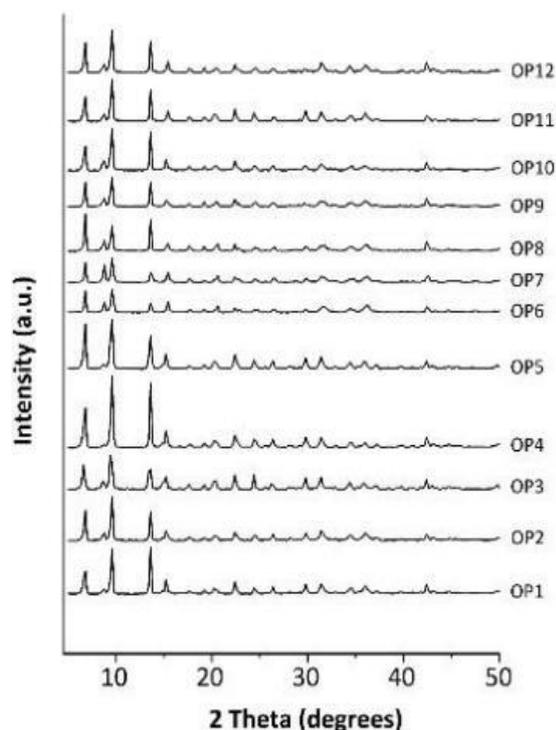
**Figure 3:** XRD of optimized formula showing characteristic peaks of MOF-5
