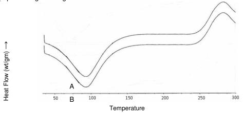
Figure 3: DSC spectra of chitosan (A) and chitosan acetate (B)
