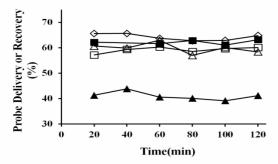
Fig 3: Delivery and recovery of puerarin in different solutions. **Key:**  $\blacksquare$  = delivery of solution 1;  $\square$  = recovery of solution 1;  $\triangle$  = delivery of solution 2  $\triangle$  = recovery of solution 2;  $\Diamond$ = recovery of solution 3. **Note:** Delivery of solution 2 is significantly different from delivery of solution 1 at p < 0.01 while recovery of solution 3 is significantly different from recovery of solution 1 at p < 0.01.
