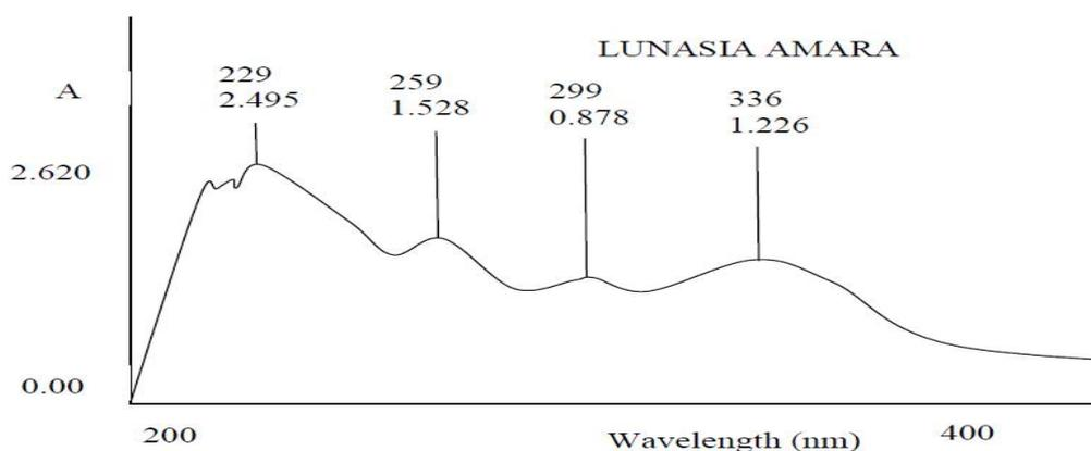
**Figure 3:** UV-Vis spectra of Beta-beta wood extract fractions
