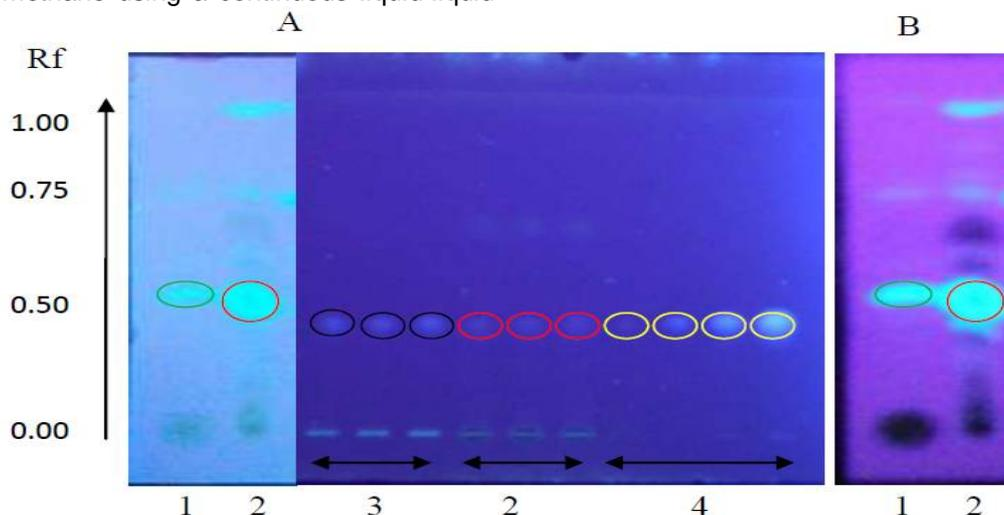
**Figure 2:** Thin-layer chromatogram: (1) Ethanol extract; (2) Dichloromethane fraction; (3) Beta-beta wood isolate; (4) Scopoletin standard; A: Observation at UV 366 nm; B: Spots seen when sprayed with KOH 10 %
