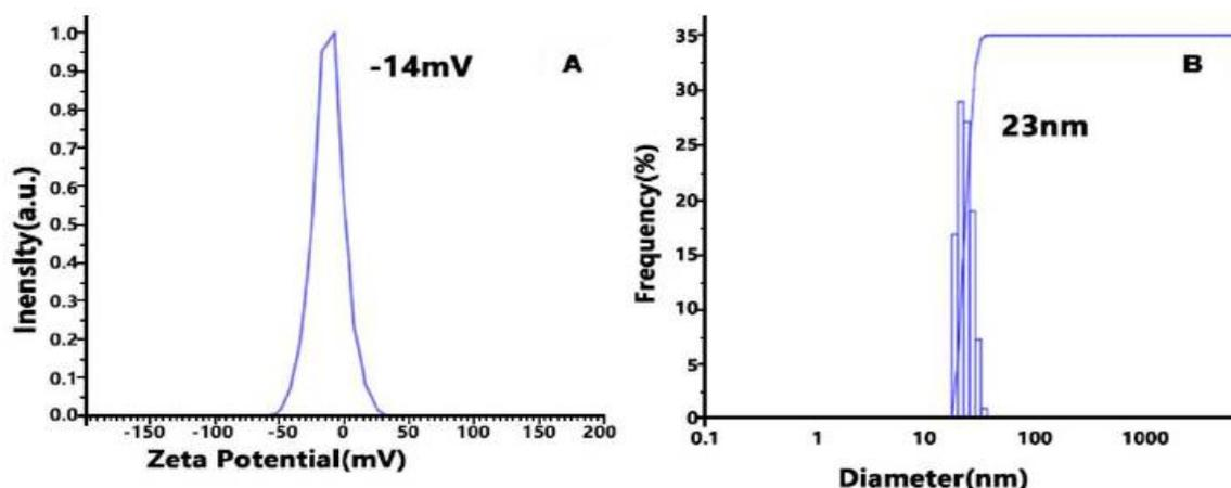
**Figure 3:** (A) Zeta potential value of TiO<sub>2</sub> NPs and (B) average size of the prepared NPs.
