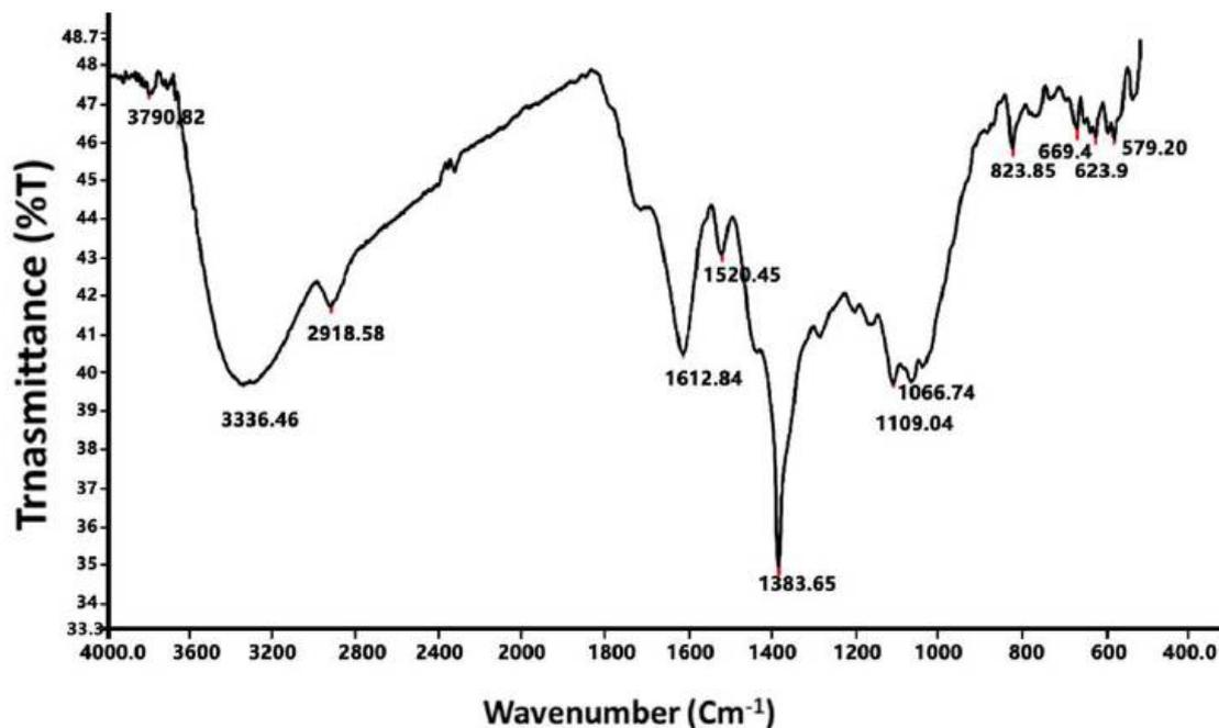
**Figure 5:** Fourier transform infrared (FT-IR) spectrum of TiO<sub>2</sub> NPs prepared using *Cinnamomum tamala* leaf extract
