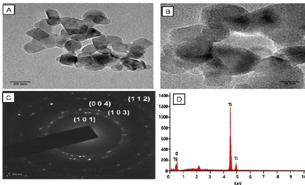
**Figure 2:** (A, B) Transmission electron microscopy (TEM) images of TiO<sub>2</sub> NPs, (C) selected-area electron diffraction (SAED) pattern of the NPs, and (D) energy dispersive X-ray spectroscopy (EDS) profile showing the elements contained in the NPs
