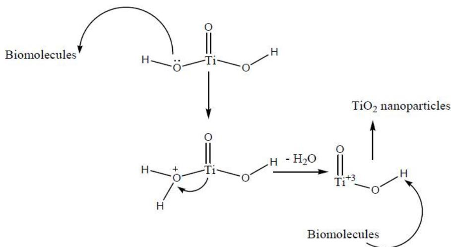
**Figure 6:** Plausible mechanism for the formation of TiO<sub>2</sub> NPs
