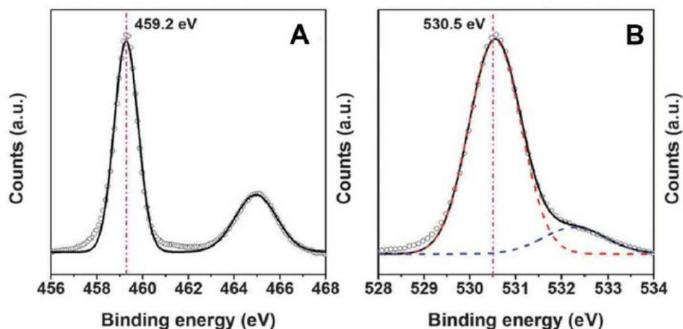
**Figure 4:** High-resolution x-ray photoelectron spectroscopy (XPS) spectra of (A) the titanium 2p peak and (B) the oxygen 1s peak of TiO<sub>2</sub> NPs
