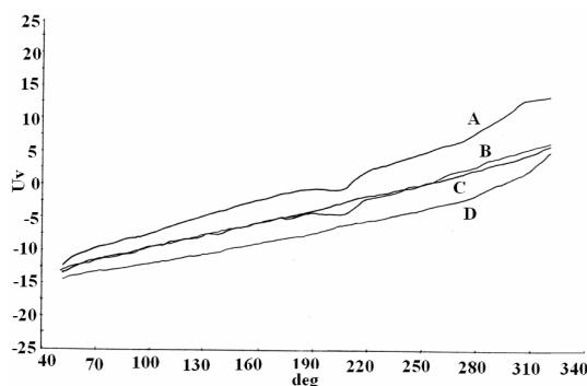
**Figure 4:** DTA thermograms of BH (A), physical mixture (B), HP-β-CD (C) and inclusion complex (D)
