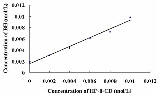
**Figure 1:** Phase solubility diagram of BH/HP- $\beta$ -CD system in water
