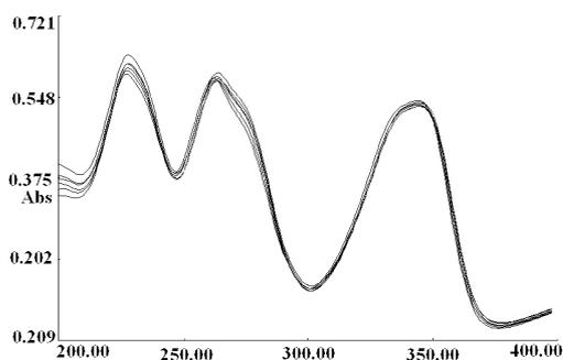
**Figure 2:** UV-visible absorption spectra of BH dissolved in HP- $\beta$ -CD solution of varying concentrations (0, 3.0, 6.0, 9.0, 12.0, 14.4 mmol/L). **Note:** The lower concentration the higher the absorption
