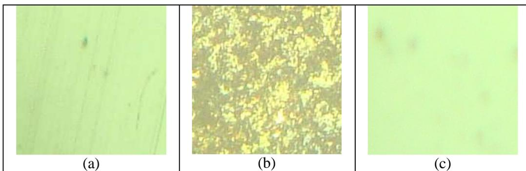
**Figure 2:** Optical microscope photographs of the working electrode (ie. carbon steel electrode) at various experimental conditions (a) Freshly polished surface, (b) After immersion in uninhibited test solution for 9 hours, (c) After immersion in inhibited test solution with inhibitor concentration: 200 ppm for 9 hours.
