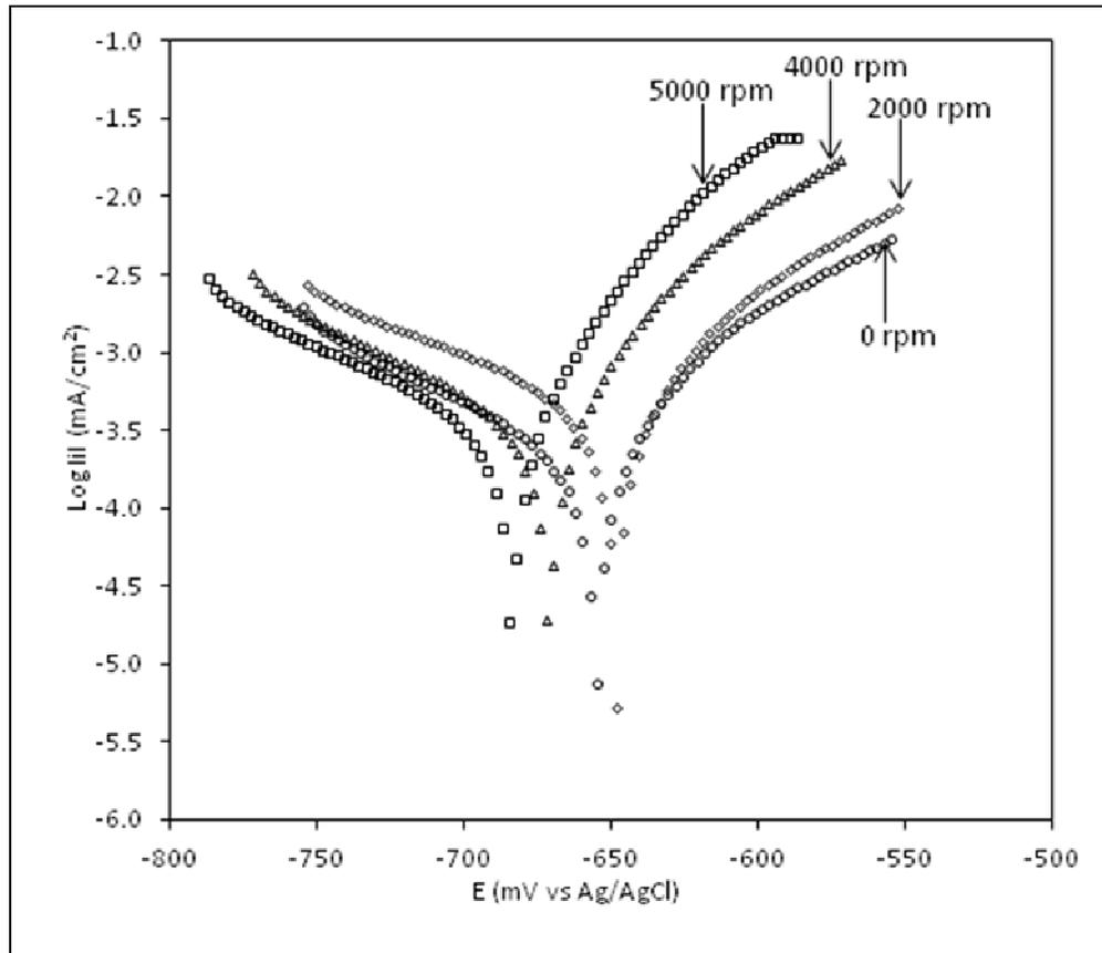
**Figure 4:** Selected polarization curves showing the performance of *Aloe Secundiflora* at different rotation speeds.
