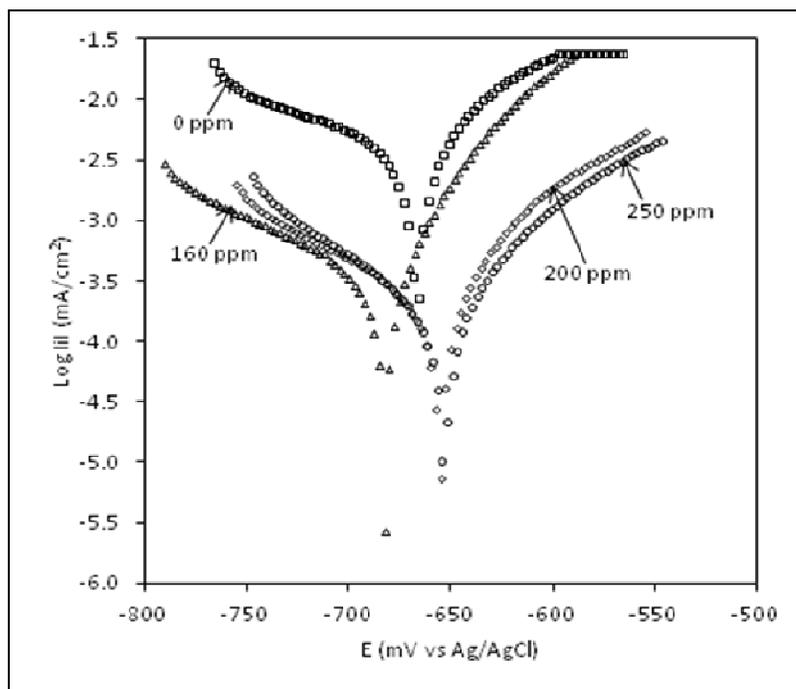
**Figure 3:** Selected polarization curves showing the performance of *Aloe Secundiflora* at different inhibitor concentrations.
