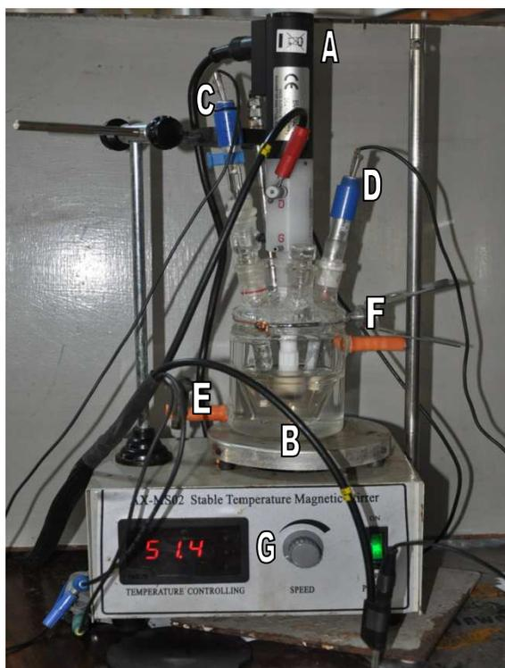
**Figure 1:** Schematic drawing of the glass cell experimental setup. (A = Rotating Disc Electrode; B = Working Electrode; C = Reference Electrode; D = Counter Electrode; E = Water in; F = Water out; G = Temperature controlling unit)
