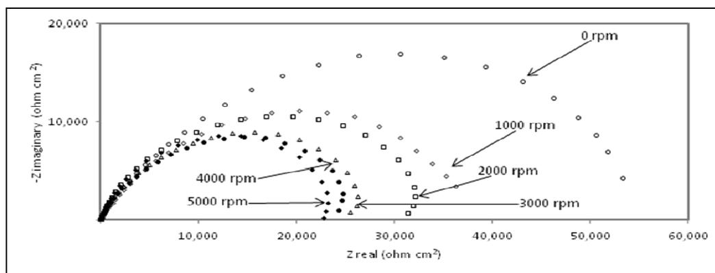
**Figure 6:** Impedance spectra in Nyquist format showing the performance of 200 ppm *Aloe Secundiflora* at different rotation speeds.
