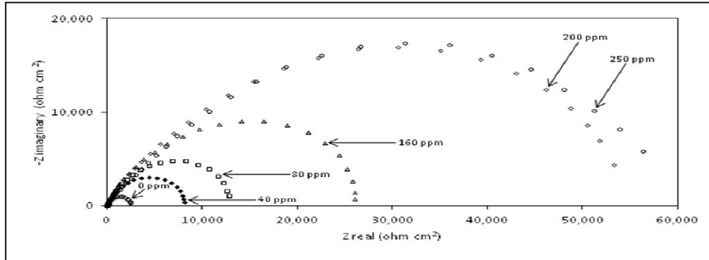
**Figure 5:** Impedance spectra in Nyquist format showing the performance of *Aloe Secundiflora* at different inhibitor concentrations.
