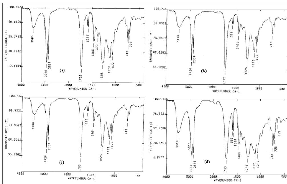
**Figure 1:** FTIR spectra of long oil alkyd resin for Re (a), N1 (b) N2 (c) and N3 (d)
