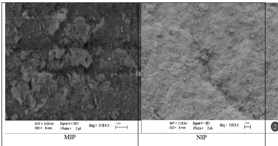
**Figure 2:** SEM micrographs MIPs and NIPs (represented by MIP4 and NIP4) showing morphology of the polymers
