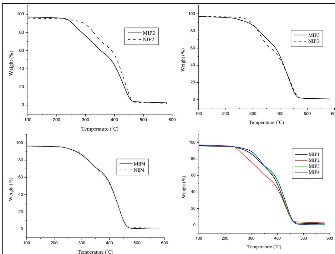
**Figure 4:** Comparison of TGA profile between MIPs and NIPs prepared in different template to monomer ratios
