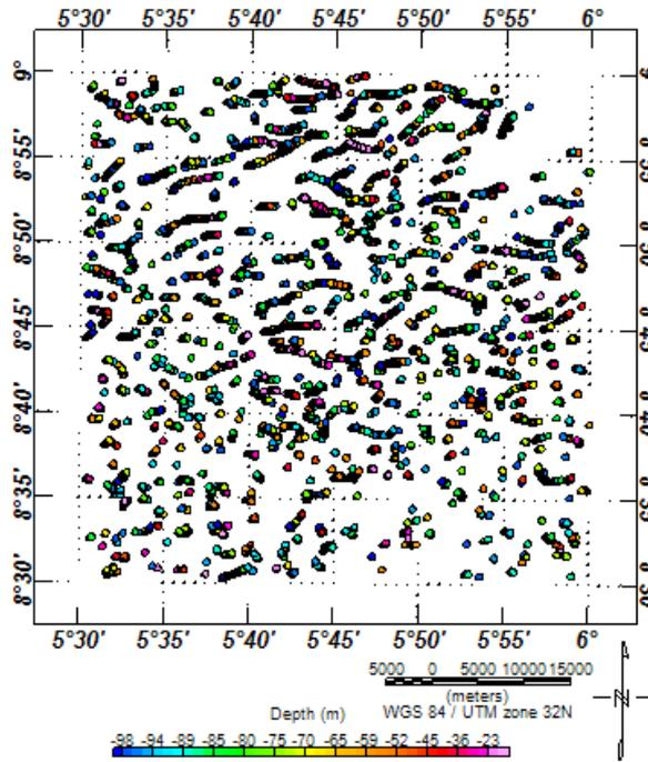
Figure 5: Magnetic (REDE) Euler Solution Map for Deep Seated Fault (SI = 0.0)
