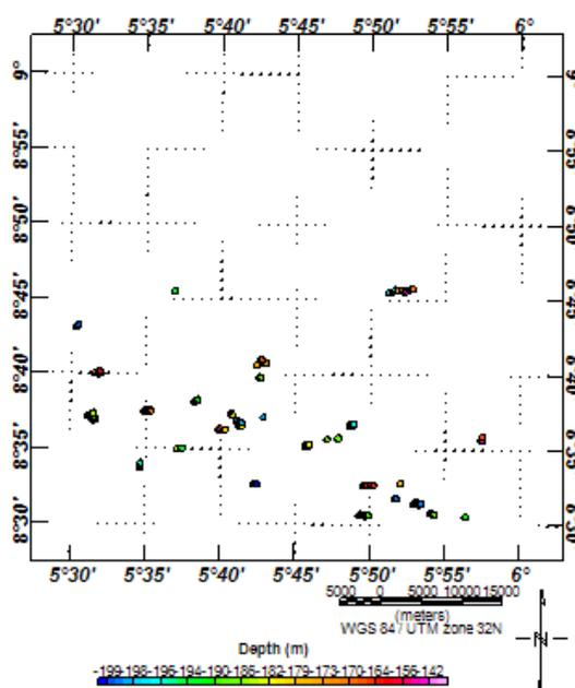
**Figure 9:** Magnetic (REDE) Euler Solution Map for Sphere (SI = 3.0)
