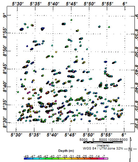
Figure 6: Magnetic (REDE) Euler Solution Map for Near Surface Fault (SI = 0.5)
