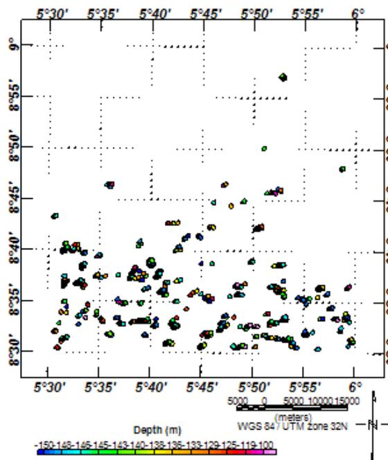
Figure 8: Magnetic (REDE) Euler Solution Map for Deep Seated Dyke/Ribbon and Sill (SI = 2.0)
