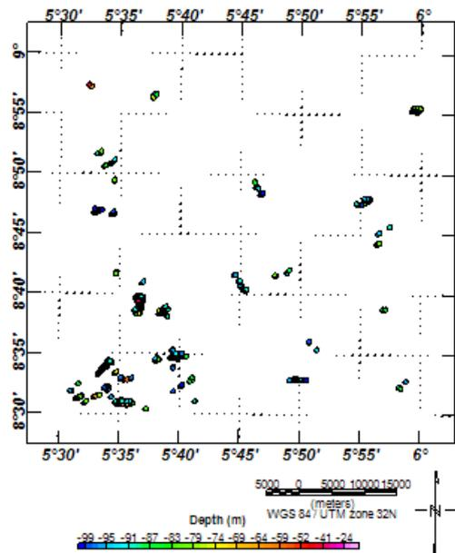
Figure 11: Pseudogravity Euler Solution Map for Ribbon/Dyke/Sill (SI = 0.5)
