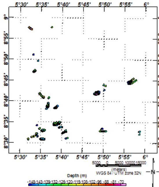
Figure 12: Pseudogravity Euler Solution Map for Dyke and Pipe (SI = 1.1)
