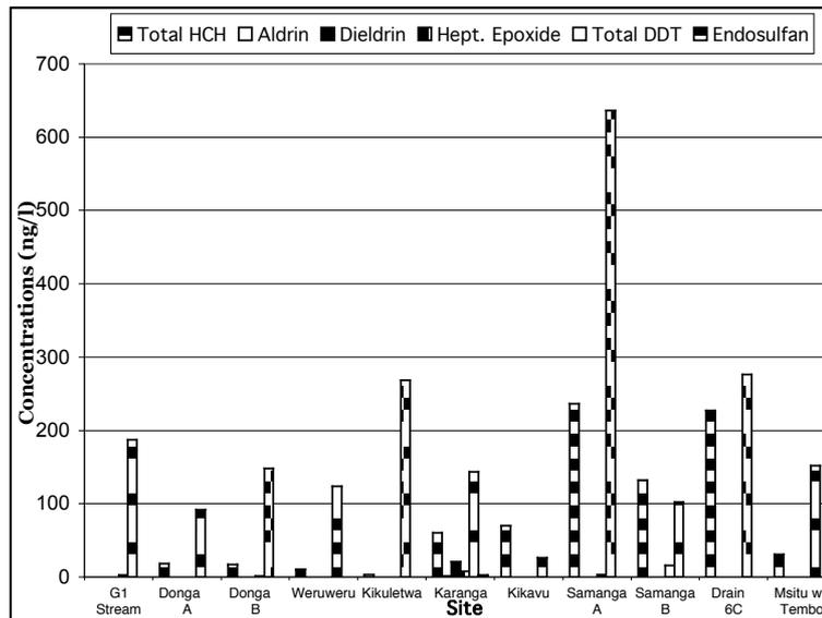
Figure 3: Pesticide residue concentrations in dry season samples
